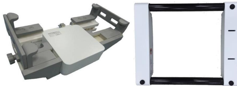
Figure 3-8 Magnetic Field Generator
