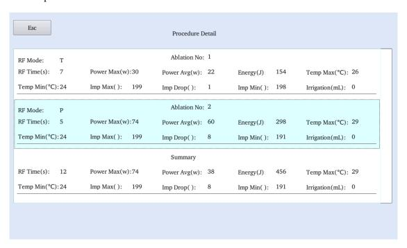
Insert the USB storage device on the back of the RF generator and check the procedure needs to be exported on the list, press "export" to complete the data export, and a progress indication is given during the export process. The format of the exported data is PDF, it could review in the PC.
